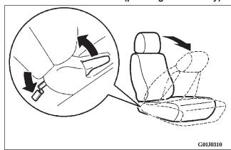
To permit rear seat entry or exit, the front seatback will fold down and the seat will move forward when the seatback lock lever is pulled up or when the pedal in back of the front passenger seat is depressed.
